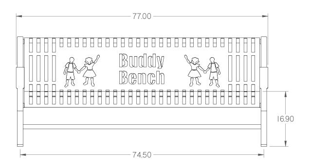
MATERIAL SPECIFICATIONS: 13 GA Mild Steel - Perferated Seating Surface 11 GA & 7 GA Mild Steel - Seating Support Frame Cast Aluminum Leg Frames
